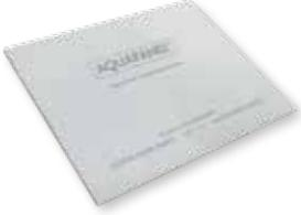
Aggregated Portland cement board with coated glass fibre mesh embedded in back and front surfaces. The ends are square cut and the edges reinforced and finished smoothly (EasyEdge™).
